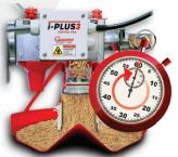
When the feed drops below the infrared sensors, the auger will re-start automatically after a 60 second delay.
