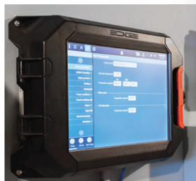
Pair your Commander fans with an EDGE® controller for complete system management and remote access capability.
