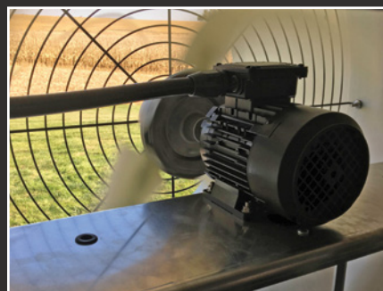
High performance, permanent magnet motor runs cool to the touch and supplies constant torque to the propeller.
