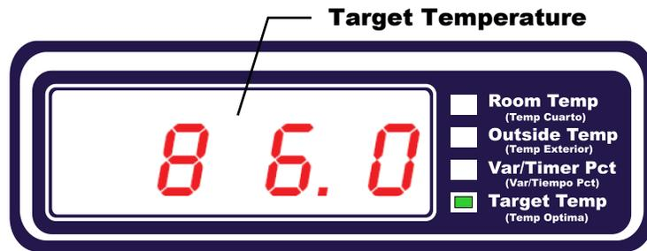
To adjust these settings, press the mode button until you see the setting you want to adjust. Then, use the + button to raise the value and the - button to lower the value. When you are finished setting a new value, either press the mode button again, or do nothing, and the system will return to normal operation within a few seconds.
