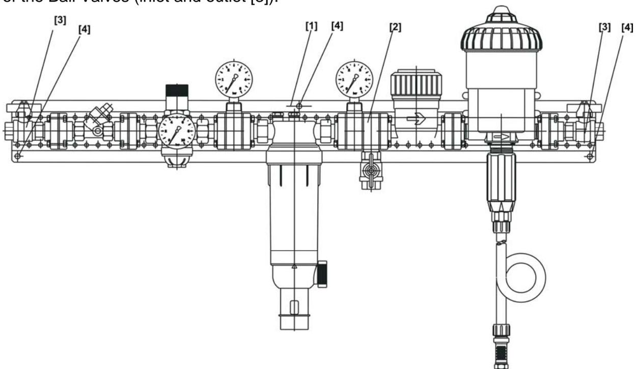
The Main Water Supply is secured horizontally to the point specified in the plans. Please observe the flow direction (arrow on the Water Meter) when connecting to the water supply!
