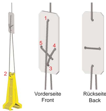
The LUBING adjusting and holding sheet metal is mounted as indicated in the above diagram. The wire hanging from the ceiling is pulled approx. 50 cm through drill hole 1. Then the rope has to be guided through drill hole 2 in the dropper clamp for the aluminium profile. The end is pulled approx. 5 cm through drill hole 3 in the retaining panel to secure. Then it is pulled through drill holes 4 and 5 and the end laid under the wire between drill holes 3 and 4. Finish by pulling the wire taut.
