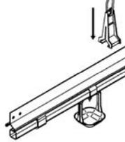
18. Secure the first suspension line to the Pressure Regulator. The suspension cables are clamped approx. 10 cm above the hanger using the adjusting and holding sheet metal.
