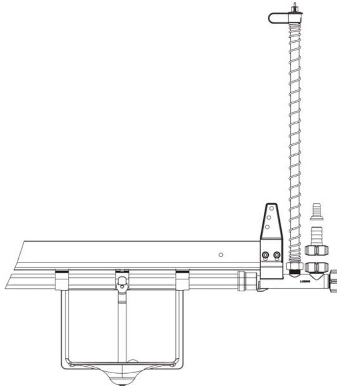
17. Clip the hanger onto the aluminium profile. The hanger are positioned beside the metal coupler.
