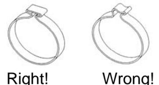
CAUTION! Aluminium carrier profiles must joint firmly to ensure good longitudinal flush along the profiles.
