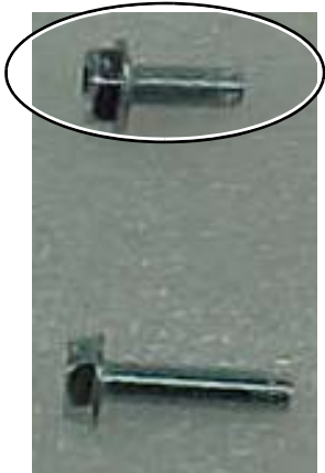
Use #10-32 x 1/2" slotted hex head type "F" screws
